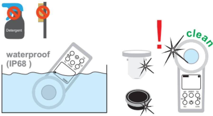
It is important to clean the device after each measurement to get rid of any reagent residues! Please ensure that the cuvette has been cleaned before each measurement (e.g. under clear water/or simply rinsing the cuvette in the pool is sufficient as long as no residues remain).
