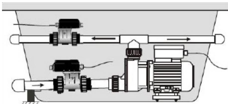
**NOTE:** The connection pipe/hose must have the same diameter as the rest of the pipe system in the spa/hot tub.
