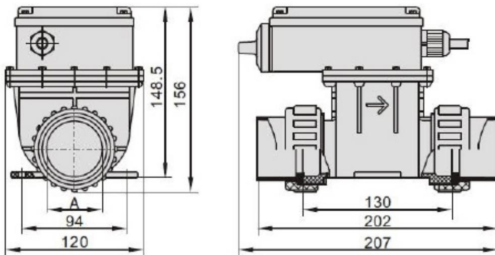
2. The heater can be connected by the system's pump intake or outlet (Fig. 2)
