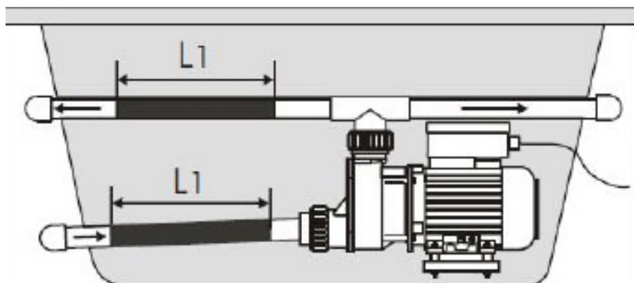
3. PVC pipe: (Fig. 3) cut a suitable piece of PVC pipe/hose from the pump's intake/outlet and mount it on the heater's fitting valve.
