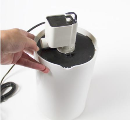
Isolate the power supply and remove the pump housing from the pool.
