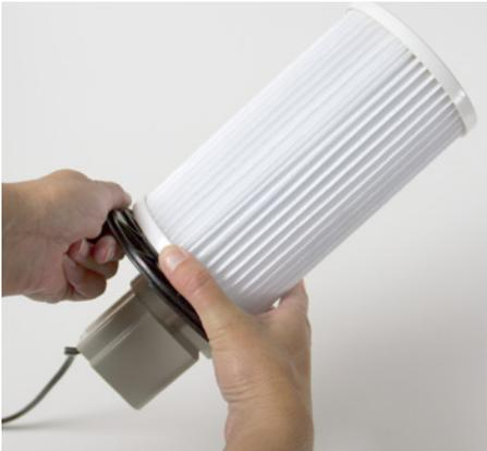
Unscrew the filter by taking hold of the bottom plastic edge and turning it anti clockwise until the filter is loose from the black mounting plate.
