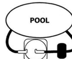
You pool and pump with 2 pcs. sun heater ( Install the heater on the returnlet from the pool , so the water runs thru the heater sand back to the pool)
