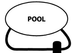
Your pool and pump with 1 pcs. sun heater ( Install the heater on the returnlet from the pool , so the water runs thru the heater and back to the pool)
