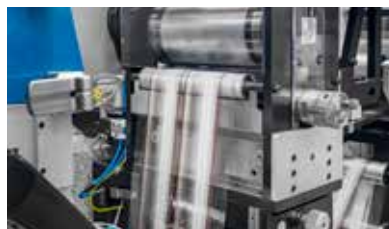
Semi-rotary die-cutting unit with compensator.
