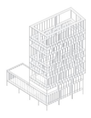
The enveloping facade-grid is a light structure defining the vertical mini-communities of various housing typologies, and mediating the scale of the tower between the urban and the human
